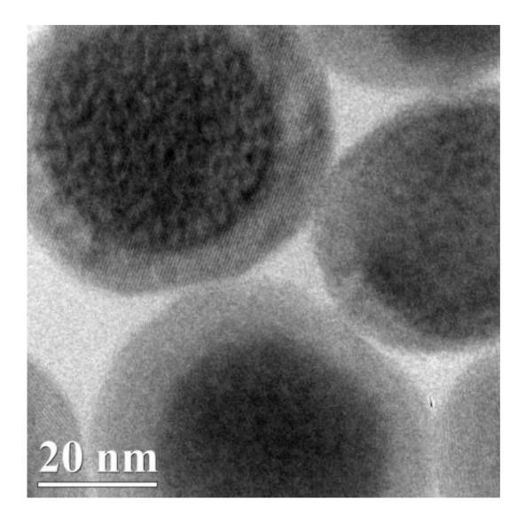
This transmission electron microscopy image shows the nanoparticles, which consist of a core that glows blue when struck by near-infrared light, and an outer fabric of porphyrin-phospholipids (PoP) that wraps around the core. Credit: Jonathan Lovell
