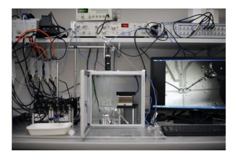
Laboratory with micro-fluidic system for serial studies of cell membranes at the Institute of Physical Chemistry of the Polish Academy of Sciences in Warsaw, Poland. On the right microscope image of two contacting droplets in the measuring chamber; visible micro-electrodes (two dark diagonal lines) for measuring currents flowing through the membrane. Credit: Polish Academy of Science, Grzegorz Krzylewski
