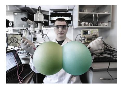
A bilayer lipid membrane is formed at the junction of two droplets. The phenomena occurring on it can be analyzed by the appropriate electrodes. The idea of constructing a microfluidic system for serial studies of cell membranes is presented by Ph.D. student Tomasz Kami?ski from the Institute of Physical Chemistry of the Polish Academy of Sciences in Warsaw, Poland. Credit: IPC PAS, Grzegorz Krzy?ewski
