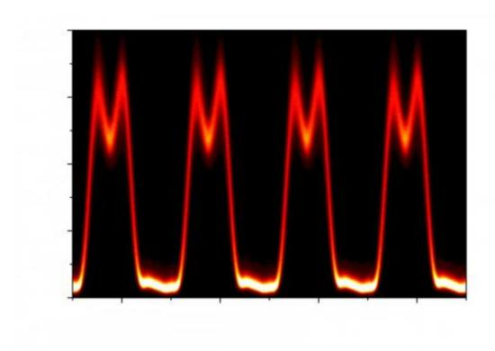
Example of custom-shaped pulses at 100-GHz repetition rate. Credit: University of Southampton
