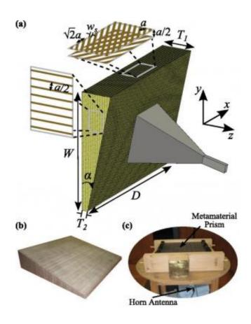
(a) Illustration of the metamaterial prism, consisting of a stack of circuit boards and metallic strips, illuminated by a horn antenna. (b) Photo of the fabricated metamaterial prism prototype. (c) Photo of the experimental setup. Credit: Morgado, et al. ©2014 AIP Publishing
