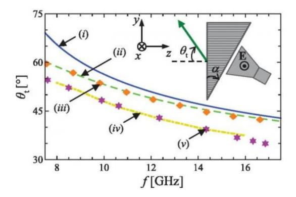
In the metamaterial, as the frequency of light increases, the transmission angle of the light decreases. This means that longer wavelengths are more refracted than shorter wavelengths, which is the opposite of what happens in conventional materials. Credit: Morgado, et al. ©2014 AIP Publishing
