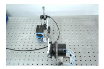
A capacitance gauge (top left) measures the accuracy of a micromanipulator system (bottom right), which is controlled by an enhanced analytic forward model. Credit: A\*STAR Institute for Infocomm Research
