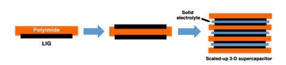
A schematic shows the process developed by Rice University scientists to make vertical microsupercapacitors with laser-induced graphene. The flexible devices show potential for use in wearable and next-generation electronics. Credit: Tour Group/Rice University
