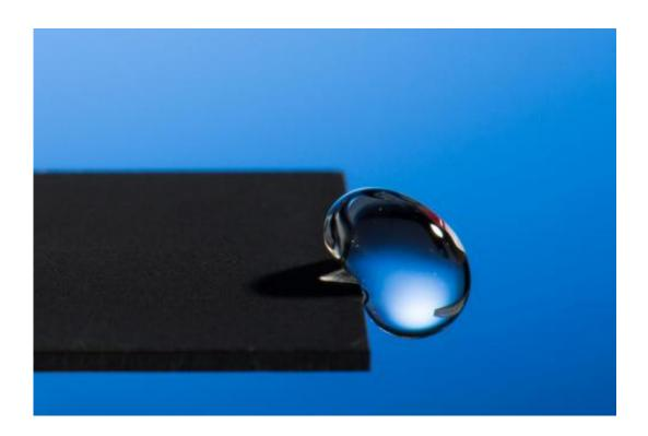
University of Rochester's Institute of Optics Professor Chunlei Guo has developed a technique that uses lasers to render materials hydrophobic, illustrated in this image of a water droplet bouncing off a treated sample. Credit: J. Adam Fenster/University of Rochester
