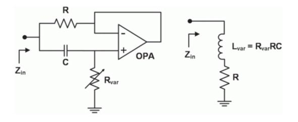
The gyrator circuit (left) and its LR equivalent (right) to eliminate saturation in the detector
