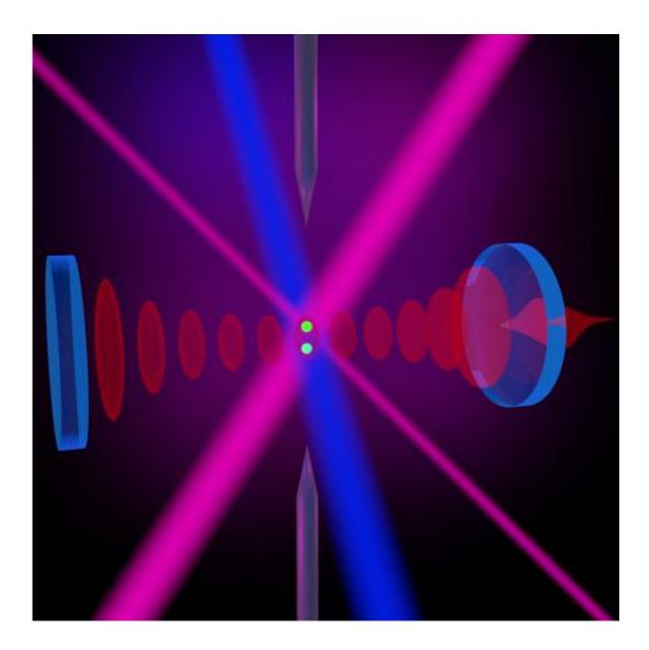
Two particles are positioned between highly reflective mirrors and entangled with one another by means of a laser. Additional lasers encode quantum information in the ions and then transfer the information to a single photon. Credit: U. Innsbruck
