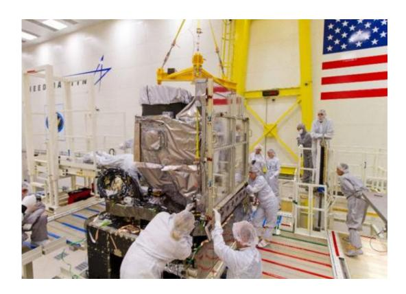
The GOES-R Advanced Baseline Imager (ABI) is installed onto the GOES-R spacecraft at Lockheed Martin in Littleton, Colorado, on October 13, 2014. Credit: Lockheed Martin
