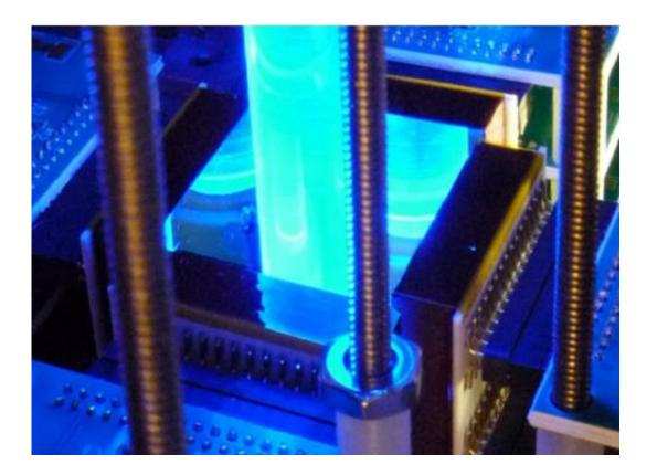
The X-ray beam enters the scattering slab (blueish glow) from the top. The Xrays are scattered in the slab with a scattering distribution characteristic depending on the polarization properties of the incoming beam. The scattering distribution is measured with semiconductor X-ray detectors surrounding the scattering slab on all four sides. The digitized signals are received through the readout electronics that are attached at the back-side of each detector. Credit: JAI
