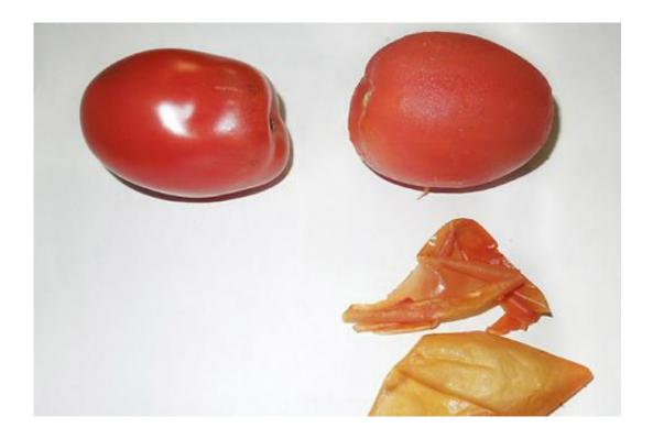
Tomatoes before and after peeling using an infrared heating system developed by ARS scientists and their industry and university colleagues. Credit: Z. Pan Laboratory
