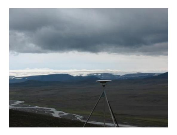
This global positioning satellite receiver is part of Iceland's network of 62 such receivers that geoscientists are using to detect movements of the Icelandic crust that are as small as one millimeter per year. Langjökull glacier can be seen in the background. Credit: Richard A. Bennett/ University of Arizona
