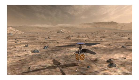
A proposed helicopter could triple the distances that Mars rovers can drive in a Martian day and help pinpoint interesting targets for study. Credit: NASA
