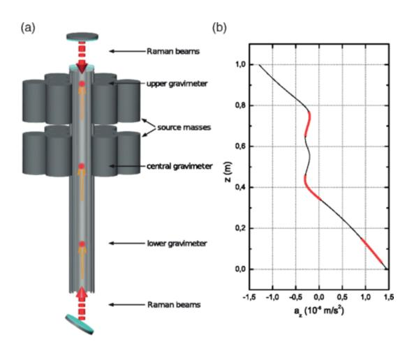
(a) Scheme of the experiment. (b) Gravitational acceleration along the symmetry axis (az) produced by the source masses and the Earth's gravity gradient. Credit: *Phys. Rev. Lett.* 114, 013001
