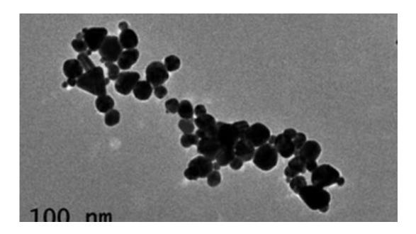
Microscopic view of microplasma-gold nanoparticles on a new, highly sensitive, test strip that enables early detection of heart attacks.
