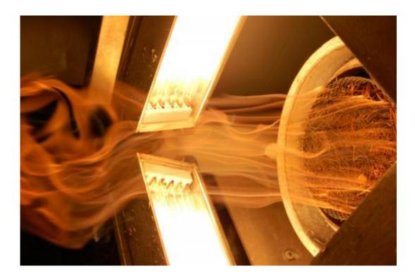
Fire propagation apparatus recreating the impact induced thermal pulse at the Cretaceous-Palaeogene (K-Pg) boundary. Halogen lamps are delivering the thermal radiation. Credit: University of Exeter
