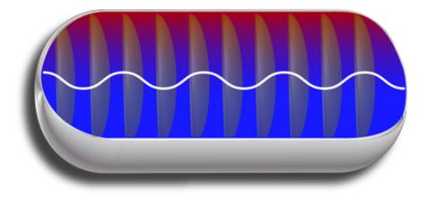
Schematic diagram of a gas-filled pressure vessel. The red-to-blue shading represents the temperature gradient in the gas, with the higher (red) temperatures near the top. The ovals represent a standing sound wave; its frequency is mostly determined by the average temperature of the gas. The wavy line represents a resonant electromagnetic wave; its frequency is mostly determined by the length of the tank. Wavelengths are not to scale.
