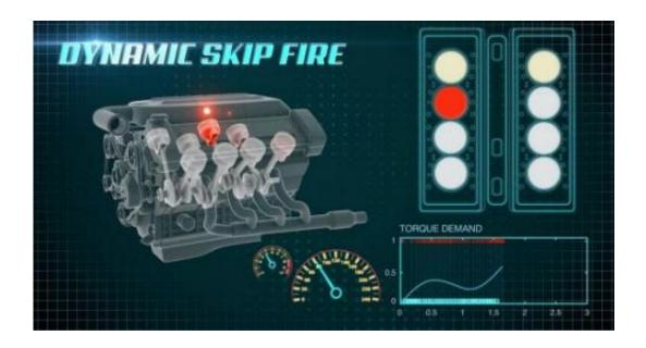
Tula Technology's Dynamic Skip Fire (DSF) technology integrates advanced digital signal processing with sophisticated powertrain controls to create a software-based approach to variable displacement engines. The result makes the most of vehicle fuel economy across a wide range of driving conditions. DSF could be deployed in future gasoline engine-powered General Motors' vehicles.
