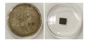
The image on the left shows the neat GO film, which disintegrated in water. The contaminated film on the right remains stable.
