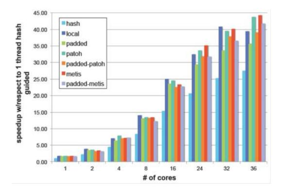
Strong scaling results on Tilera for the Europe data set using guided scheduling for different techniques. Speedup is relative to serial performance in Blondel et al. (2008).
