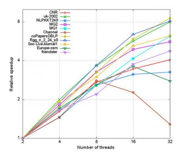
Speedup of Grappolo on a multi-core platform for different inputs. Speedups are relative to the same code using two threads.
