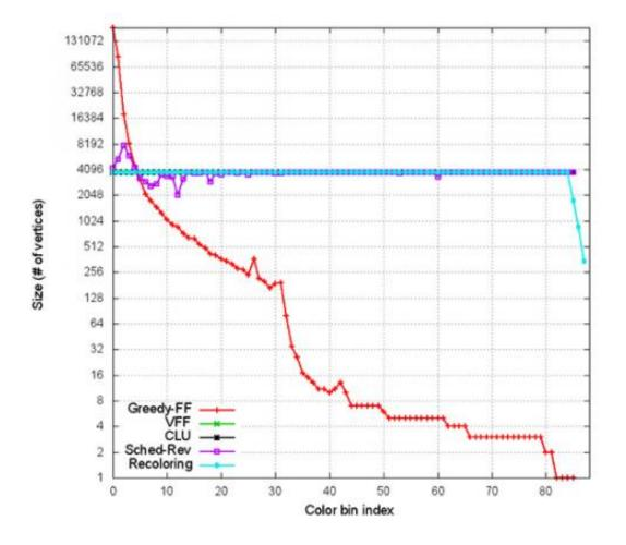
Distribution of color-class sizes for coloring computed from different heuristics. The red line represents the original algorithm with significant variance. All other lines are based from the new heuristics: the flatter the line, the better.
