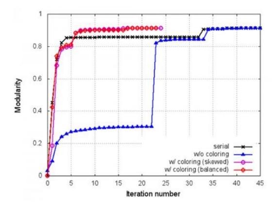
Evolution of modularity gain as the algorithm progresses (iterations along X axis) for CNR data set. Parallel implementation without coloring converges slowly.
