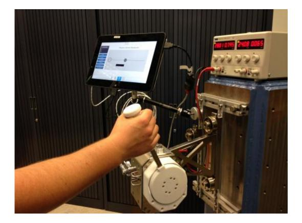
The Haptics-1 experiment – seen here during testing – comes down to a deceptively simple-looking lever that can be moved freely to play simple Pong-style computer games. Behind the scenes, a complex suite of servomotors can withstand any force an astronaut operator might unleash on it, while also generating forces that the astronaut will feel in turn, just like a standard video
