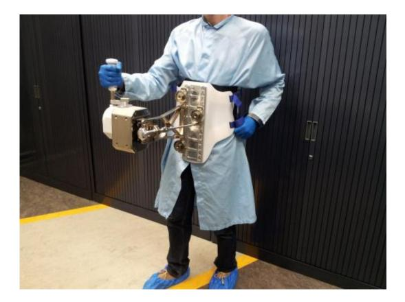
Body-mounted astronaut joystick for the Haptics-1 experiment, developed by ESA's Telerobotics and Haptics Laboratory as part of the multi-agency Meteron (Multi-Purpose End-to-End Robotic Operation Network) initiative, investigating telerobotics for space. Credit: ESA
