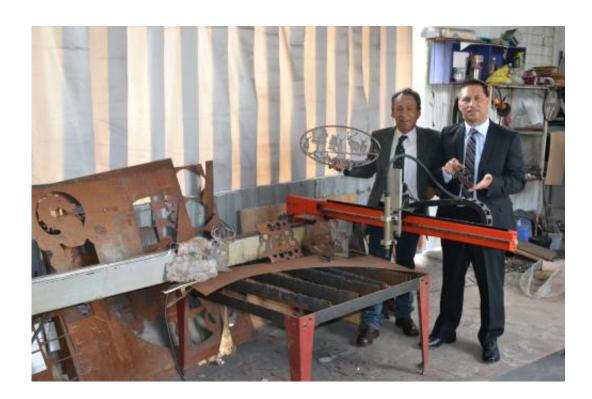
When the engineer Isaac Navarro Alcazar needed to make two-meter 3D dinosaur figures, he could not find the right tool to make the cuts. So he decided to make his own machine: an innovative, automated and efficient tool capable of making plasma cuts through plating and metal foils such as carbon steel, stainless steel and aluminum, and others.
