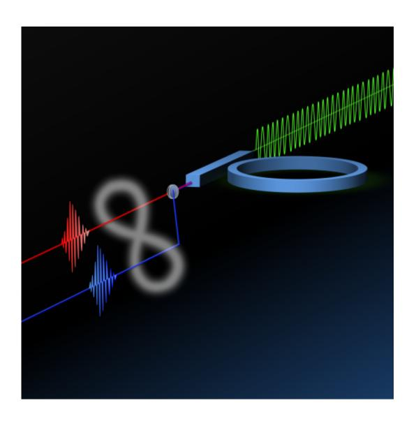
Drawing of the silicon ring resonator with its access waveguide. The green wave at the input represents the laser pump, the red and blue wavepackets at the output
