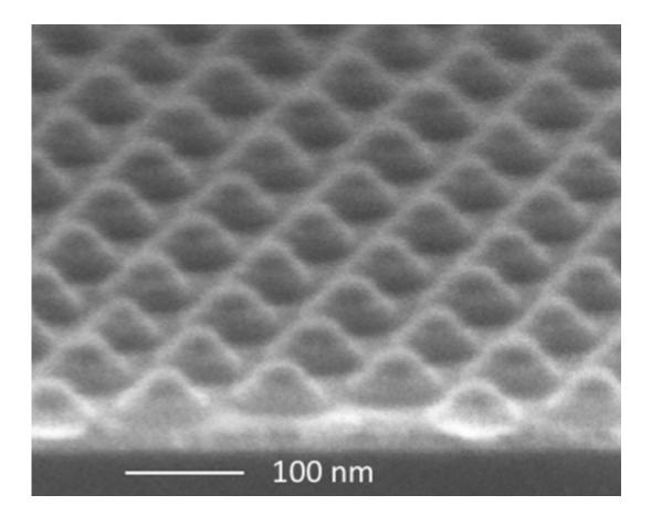
Magnetic tunnel junctions hidden under cones of tungsten used as an etch mask. The tunnel junctions were made from a film deposited by Weigang Wang's group at the University of Arizona, and patterned using self-assembled block copolymer lithography in Professor Caroline Ross' group.
