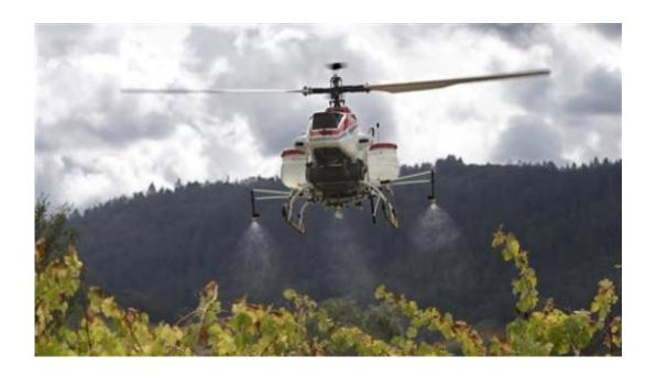
In this Wednesday, Oct. 15, 2014 photo, the Yamaha RMax unmanned helicopter sprays water over grapevines during a demonstration of its aerial application capabilities at the University of California, Davis' Oakville Station test vineyard in Oakville, Calif. Researchers at UC Davis have been studying the effectiveness of the drone's ability for spraying pest control and nutritional materials on the test vineyard in California's Napa Valley. (AP Photo/Rich Pedroncelli)
