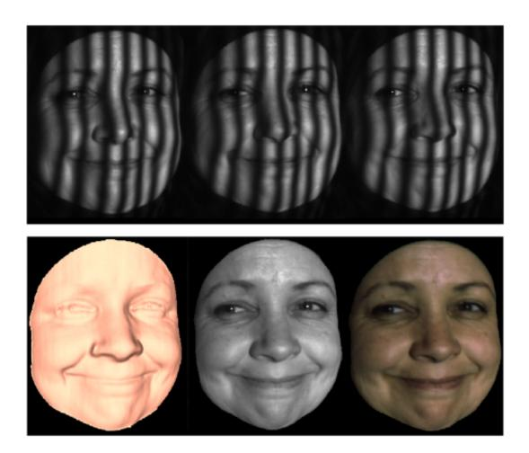
Researchers have designed a program to generate 3D imagery from the projection and digitization of binary data that allows reconstruction of
