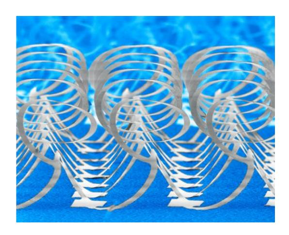
3-D microstructures of device-grade silicon formed using concepts similar to those in children's 'pop-up' books. The images correspond to colorized scanning electron micrographs. The silicon has a thickness of 2 microns. Potential applications range from battery anodes, to solar cells, to 3D electronic circuits and biomedical devices. Credit: John Rogers, University of Illinois
