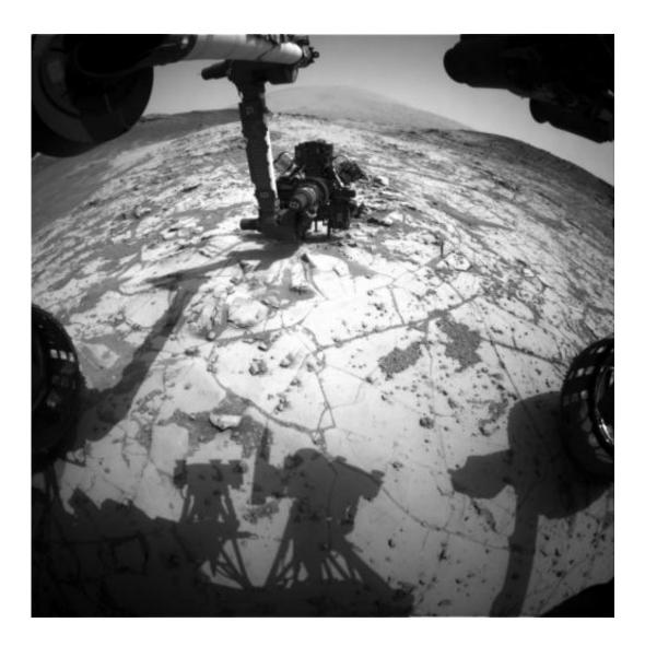
This view from the wide-angle Hazard Avoidance Camera on the front of NASA's Curiosity Mars Rover shows the rover's drill in position for a mini-drill test to assess whether a rock target called "Mojave" is appropriate for full-depth drilling to collect a sample. It was taken on Jan. 13, 2015. Credit: NASA/JPL-
