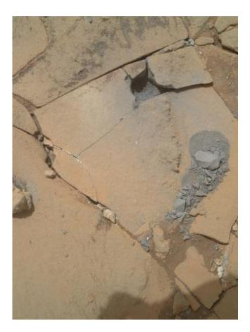
This Jan. 13, 2015, view from the Mars Hand Lens Imager on NASA's Curiosity Mars rover shows outcomes of a mini-drill test to assess whether the "Mojave" rock is appropriate for full-depth drilling to collect a sample. Cracking of the rock has made freshly exposed surfaces available for inspection. Credit: NASA/JPL-Caltech/MSSS
