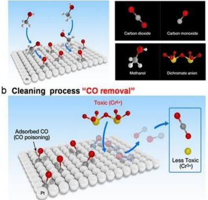
Schematic diagrams of CO poisoning removal process using Cr(VI)
