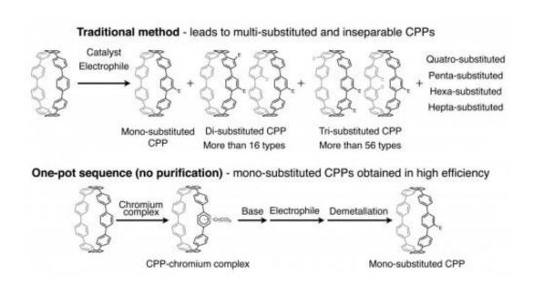
Route to substituted CPPs -- the traditional method and a one-pot sequence (this work). Credit: ITbM, Nagoya University
