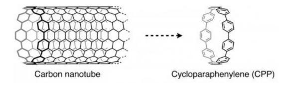
Cycloparaphenylene as a segment of a carbon nanotube. Credit: ITbM, Nagoya University
