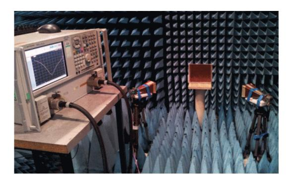
The testing rig in an anechoic chamber at QUB. Even with large incident angles, the FSS absorber is an effective RAM.
