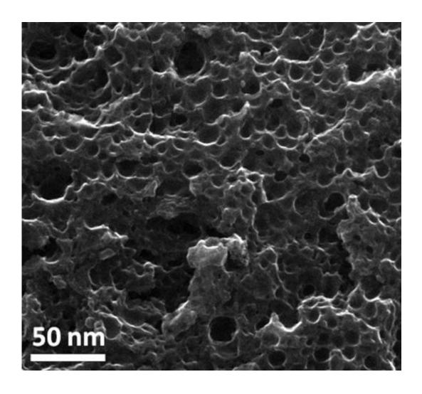
A scanning electron microscope image shows the fine pores in a carbon material created at Rice University to capture carbon dioxide from production streams at natural gas wellheads. The material sequesters carbon dioxide molecules at normal wellhead pressures and lets them go when the pressure is released. Credit: Tour Group/Rice University
