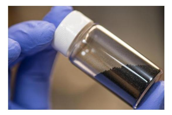
Each grain of a powder drawn from asphalt has the ability to capture more than its own weight in carbon dioxide under pressure. The material invented at Rice University is intended to separate carbon dioxide from streams at natural gas wellheads. Credit: Jeff Fitlow/Rice University
