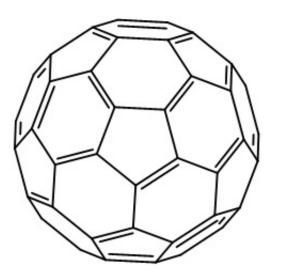
The C60 carbon ball consists of 60 carbon atoms that are placed so that the molecule resembles a nanometer-sized football. Credit: Christian Müller
