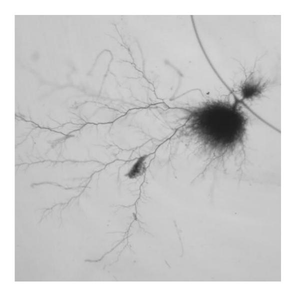
An electrical tree, which is a major electrical breakdown mechanism of insulation plastic. Fullerenes prevent electrical trees from forming by capturing electrons that would otherwise destroy chemical bonds in the plastic. Credit: Anette Johansson and Markus Jarvid
