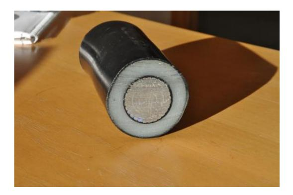
A high-voltage cable cross-section. The electrically conductive core is covered by a black protective layer, a white insulation layer of plastic and an additional
