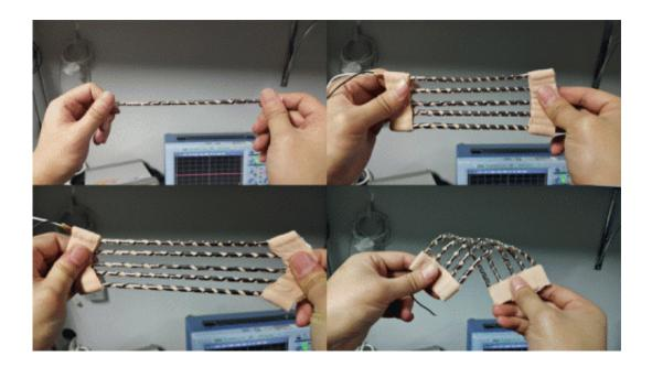
Clockwise from top left: A single structure consists of a double-helix of piezoelectric polymer strip and fabric strap around an elastic support material core; multiple structures can be connected in parallel; each can be elastically stretched to 1.6 times their rest length; it is also extremely flexible
