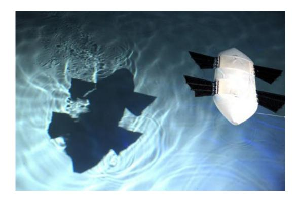
The result was the development of artificial pectoral fins integrated into a manportable, unmanned vehicle named the Wrasse-inspired Agile Near-shore Deformable-fin Automaton, or WANDA. Four side-mounted fins, two forward and two aft, provide all the propulsion and control necessary for the vehicle. Credit: U.S. Naval Research Laboratory
