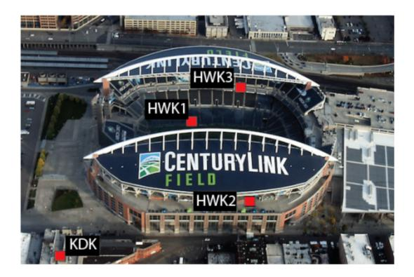
For the game, scientists will install a strong-motion seismometer labeled HWK1 at field level under the east stands, HWK2 on the second level of the west stands, and HWK3 on the upper east deck. KDK is a permanent seismometer in a building just west of the stadium. Credit: Pacific Northwest Seismic Network
