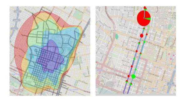
The NMC's web-based visualization tool displays simulations from DTA models. The left image shows the model's estimation of the time it takes to reach different sections of downtown during the morning peak. The right image shows
