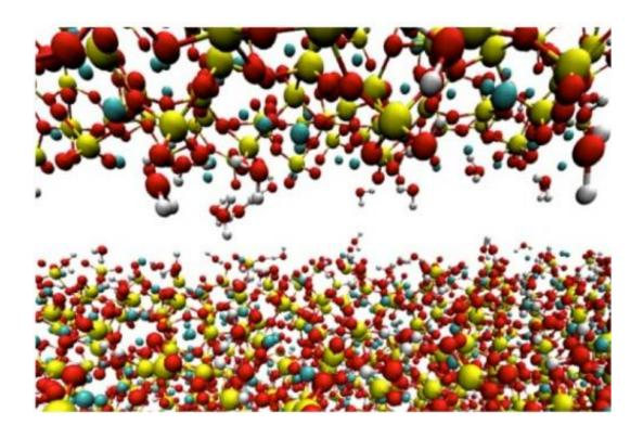
A calcium-silicate-hydrate (aka cement) tip hovers above a smooth tobermorite surface in a computer simulation by Rice University scientists. The researchers studied how atomic-level forces in particulate systems interact when friction is applied. Their calculations show such materials can be improved for specific applications by controlling the materials' chemical binding properties. Credit: Shahsavari Group/Rice University
