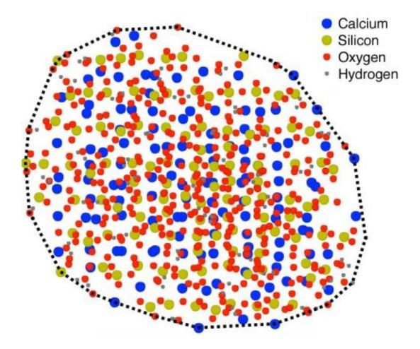
A top-down look at the tip of a virtual cement probe shows the position of atoms, dominated by calcium and silicate. Researchers at Rice University used simulations to show the chemical makeup of particulate systems affects their material strength by simulating friction with various surfaces. Credit: Shahsavari Group/Rice University
