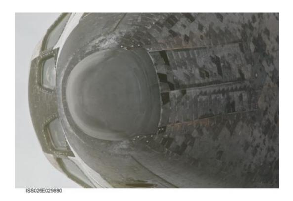
This view of the nose section of space shuttle Discovery, build of heat-resistance carbon-composites. Credit: NASA
