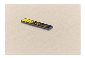
The silicon photonic chip (about 3 x 15 millimeters in size) consists of planar waveguide circuits in which photons are generated and the propagation of light is electronically controlled. The horizontal stripes of the chip correspond to different types of silicon photonics structures used to generate and control light; the features used in this experiment were located near the middle of the chip.
