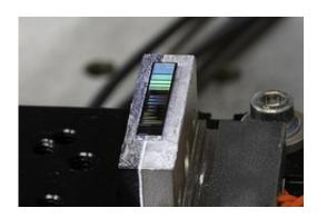
During the experiments, the silicon photonic chip was placed on a temperature-controlled stage. Fibers (not shown) were used to couple the optical pump beam to the chip at one of the cleaved facets (left side of the chip), and extract the generated photon pair from the cleaved facet at the right side of the chip.
