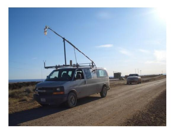
The KIT measurement instrument on board of a minivan directly measures atmospheric emissions on site with a high temporal resolution. Credit: F. Geiger/KIT
