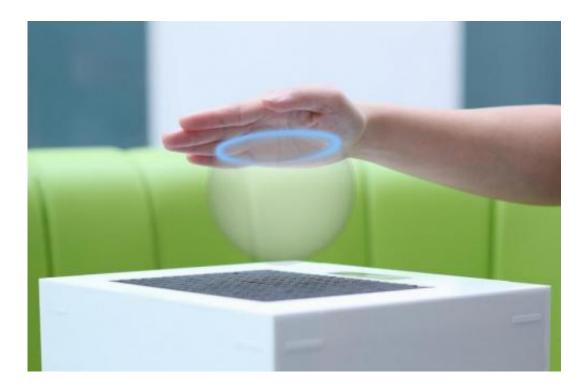
Ultrasound is focused to create the shape of a virtual sphere. Credit: Bristol Interaction and Graphics group, University of Bristol, copyright © 2014
