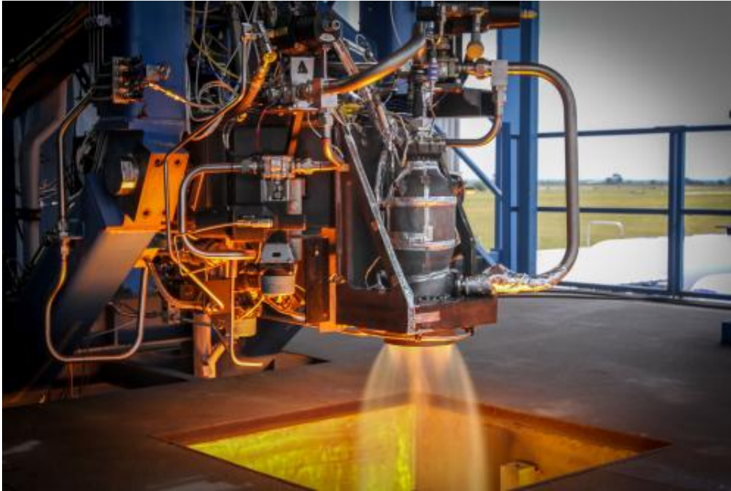
A SuperDraco thruster being tested at the Rocket Development and Test Facility in McGregor, Texas. Credit: SpaceX
