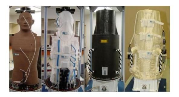
During the exposure in the open space, the MATROSHKA phantom was covered by a container imitation the shielding properties of a spacesuit. Credit: DLR
