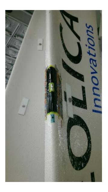
The area on the rotor blade heated by the CNTcoating remains free of ice. Credit: Fraunhofer IPA
