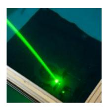
Bathymetric lidars – devices that employ powerful lasers to scan beneath the water's surface – are used today primarily to map coastal waters. At nearly 600 pounds, the systems are large and heavy, and they require costly, piloted aircraft to carry them.
