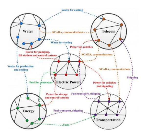
An illustration maps the interdependence of different infrastructure sectors. These complex relationships are characterized by multiple connections between infrastructure systems, feedback and feed-forward paths, and intricate, branching topologies. The connections create an intricate web that, depending on the characteristics of its linkages, can transmit shocks throughout broad swaths
