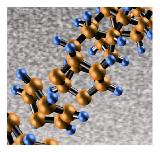
"Diamond nanothreads" promise extraordinary properties, including strength and stiffness greater than that of today's strongest nanotubes and polymers. The core of the nanothreads is a long, thin strand of carbon atoms arranged just like the fundamental unit of a diamond's structure -- zig-zag "cyclohexane" rings of six carbon atoms bound together, in which each carbon is surrounded by others in the strong triangular-pyramid shape of a tetrahedron. The threads, made for the
