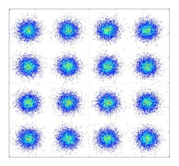
A constellation diagram of one of the mainstream modulation formats of the future system: Sixteen Quadrature-Amplitude modulation
